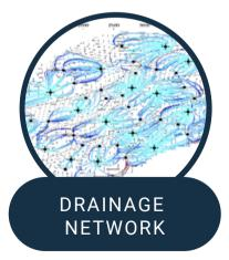
tNavigator allows visualization of drainage network lines. The thickness of these lines between wells is proportional to the value of the stream according to streamlines
