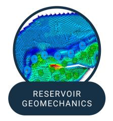
tNavigator uses a joint system of coupled equations to calculate reservoir fluid flow and geomechanical effects simultaneously.
