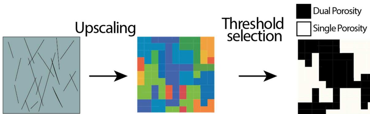
**Figure 1** Conceptual DFN model (left) is upscaled (Oda Gold method) to continuous media properties (porosity pictured in middle) and subsequently a threshold is applied to determine whether a cell is modelled as single or dual porosity. The resulting pattern corresponds to the training image used for MPS.
